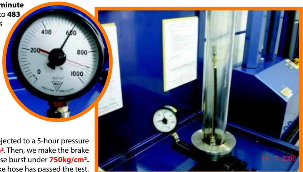
Norflex's brake hose is subjected to a 5-hour pressure amounting to **500kg/cm<sup>2</sup>**. Then, we make the brake hose burst under **750kg/cm<sup>2</sup>**. Our brake hose has passed the test.
